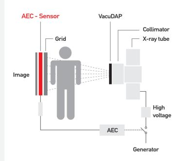
Implementation of DAP meter and AEC sensor in the beam path
